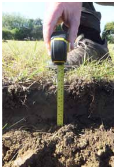
Figure 8: Ploughing depth should be less than 15cm
